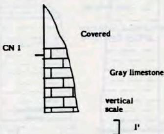
Figure 11 - Stratigraphic section of the McBryde Limestone Member at secondary location in Wilcox County (Sample CN 78 taken from 4 inch ledge of McBryde Limestone at Midway type locality)
