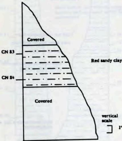
Figure 16 - Stratigraphic section of the Coal Bluff Member at Oak Hill locality in Wilcox County
