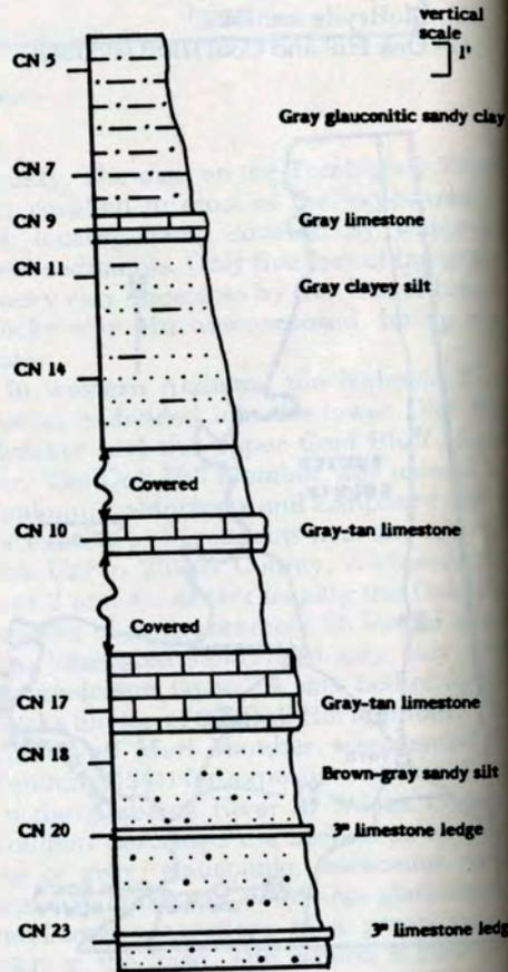
Figure 9 - Stratigraphic section of the Pine Barren Member in Wilcox County
