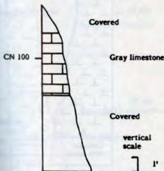
Figure 10 - Stratigraphic section of the McBryde Limestone Member at type locality in Wilcox County
